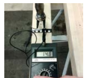
Fig. 3: Wood moisture measurement after leak-tightness test
