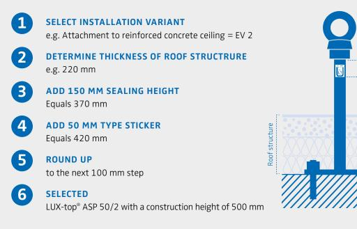
\*The diagram explains how to determine the construction height for use in the German market!
