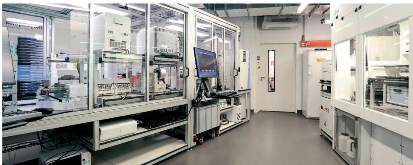
The robotic platform at Leibniz-HKI. Modules 1 and 2 are on the left, module 3 which contains a high-throughput microscope is on the right.
