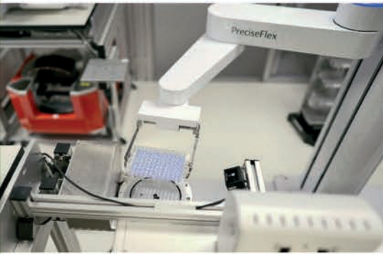
The robotic arm transports a 96-well microtiter plate to the turning table to scan the barcode. (Photos: Anna Schroll/Leibniz-HKI)
