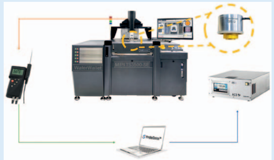
The entire system based on "ProbeSense", which is located in the wafer prober
