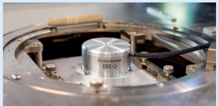
View from above of a ProbeSense fixed in the wafer prober.
