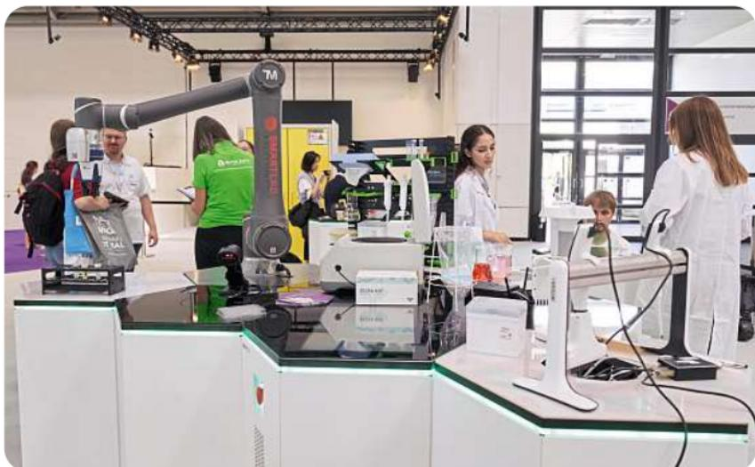
One of the highlights of the analytica special show Digital Transformation is the autonomous laboratory robot Kevin, which especially takes over routine tasks from laboratory staff. Kevin can, for example, transport samples and supply systems with reagents, pipette tips, and many other items. The mobile helper was developed at the Fraunhofer Institute for Manufacturing Engineering and Automation (IPA) and is now being prepared for series production by the United Robotics Group.
