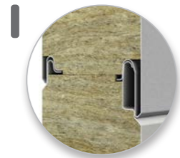
TRIMOTERM FTV HL JOINT (HIDDEN FIXING)
