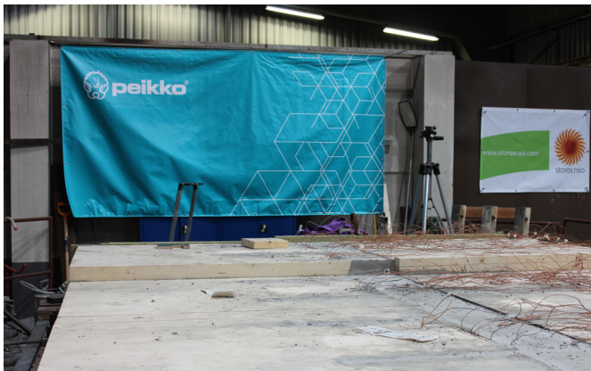
Figure 4. Specimen for the two-hour charring test without loading. CLT 200 L5s and CLT 280 L7s timber slabs were placed on the DELTABEAM® Composite Beam ledges or downstands. DELTABEAM® and the CLT 200 L5s slabs had equal depth.
