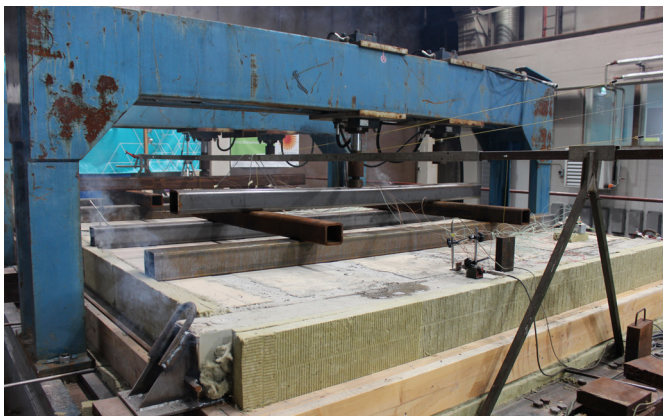
Figure 7. Specimen for the 90-minute fire test with loading. The load arrangement simulated DELTABEAM® and CLT slab structure with 8 m CLT span, 1.7 kN/m 2 permanent load and 5 kN/m 2 live load ( \psi_1 = 0.7 ). The defined factor \psi_1 is the same as used in congregation areas, shopping areas, and F traffic areas.
