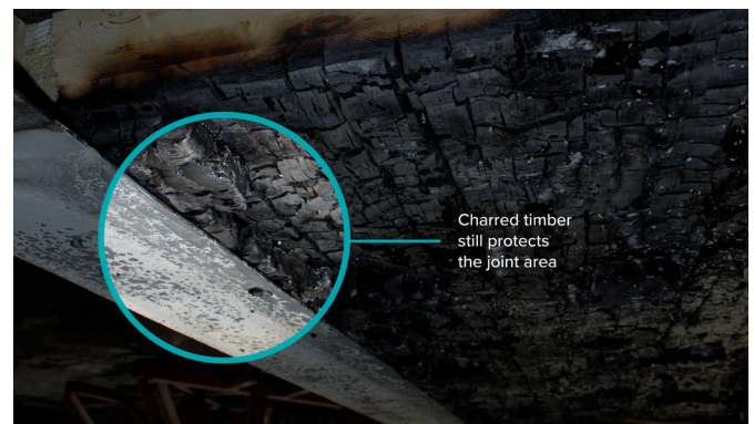
Figure 3. Specimen from below after 90-minute loaded fire test.
