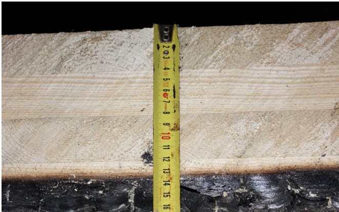
Figure 10. Charring in the middle of the CLT span.
