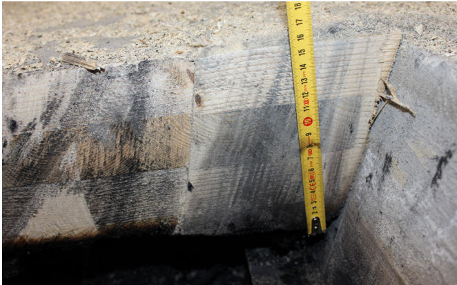
Figure 9. Charring in the DELTABEAM® and CLT slab joint, next to the joint concrete.
