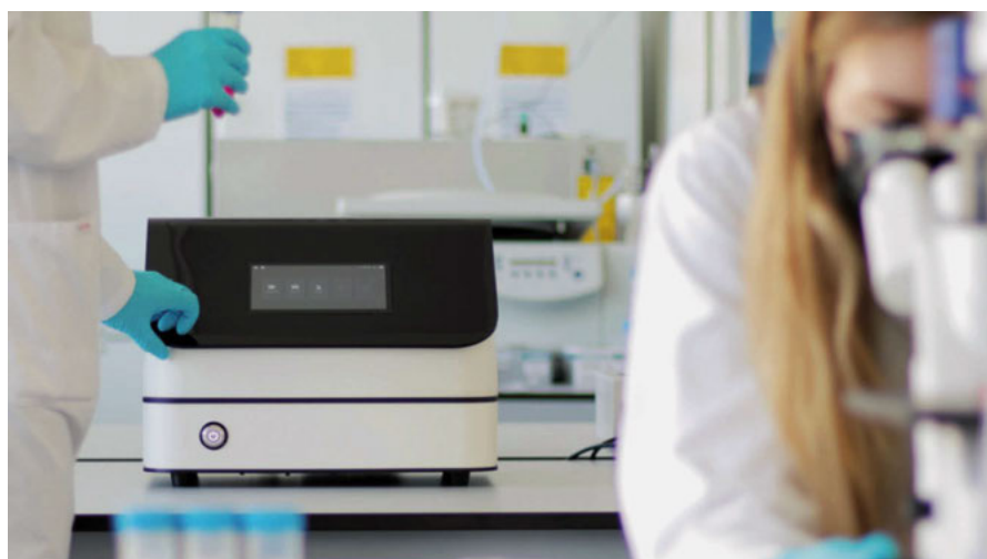
The Organicer: With this platform technology, organoids and other 3D cell based model systems can be analysed and sorted in high throughput to enable automation. (Photo: Fraunhofer IPA)
