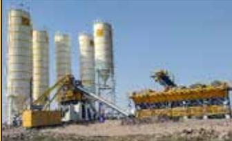
Stationary Concrete Batching Plant
