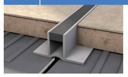
The expansion joint profile under tiling is made of coextruded hardened PVC with narrow and nonperforated bases. It is designed for use in areas with moderate loads as well as outdoor areas.
