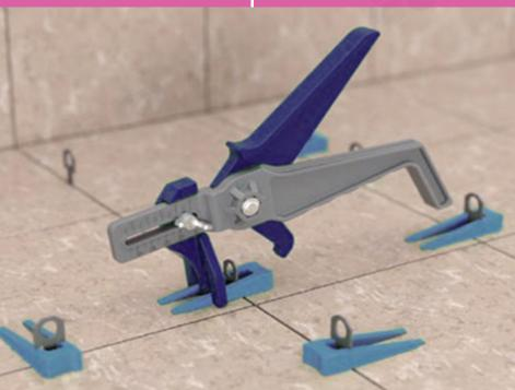
ACARA levelling pliers designed for precise levelling of tiles using PROFI system. They work on the principle of pushing the wedge around the clip until the tiles are levelled. The product prevents the tiles from shifting, which ensures that perfect joints are maintained. The ergonomic and durable design of the pliers makes the whole installation easier and faster.
