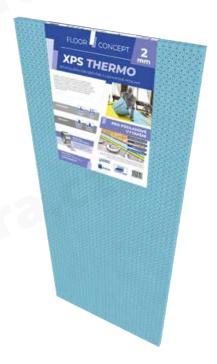
This underlayment is made of extruded polystyrene with a grooved surface. Thanks to its special design, it can be used in rooms with underfloor heating. According to the regulations, it is 2 mm thick and it is also available in rolls or sheets. It provides optimal heat conduction while maintaining the advantages of other XPS pads owing to its thick grooves, perforations on the surface, reduced thickness, and increased density.
