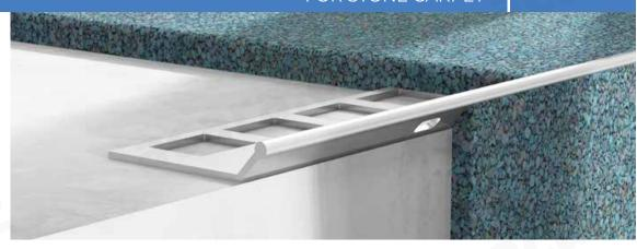
This aluminium profile has an ideal angle (135°), meaning that once the stone carpet is installed and applied, a nice detail is achieved in the form of a thin, cleaned edge. This trim also has holes along the profile to ensure an escape of water vapour or water.
