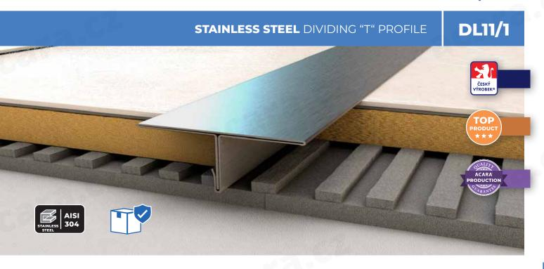
The stainless steel dividing "T" profile is used to connect two different or identical surfaces. It is installed at the end of the laying process between two adjacent floors placed at the same level. The stainless steel dividing "T" profile protects the outer edge of the floor covering. The construction of this profile with the lower vertical part of the arrowhead allows excellent anchoring with silicone or adhesive.
