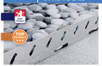
The trim is designed to hold the roof layers against sliding, to cover the front of the roof structure when viewed from below or from the side, or to separate roof sections with different layer compositions. It is available in heights of 45, 60, 80, 100 and 130 mm.
