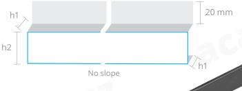
The connecting profile for a connection to the wall from the EXCELLENT series is used as a perfect straight transition from the lowered floor to the surrounding wall. The corresponding length is cut to fit between the side profiles.
