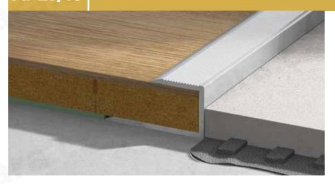
The AP27/10 trim is ideal for clean connections or terminations of laminate floors. The wide visible edge overlaps the edge of the floor which is necessary for the floor to expand. AP27/10 profiles are available in high quality aluminium in a range of different anodised shades.
