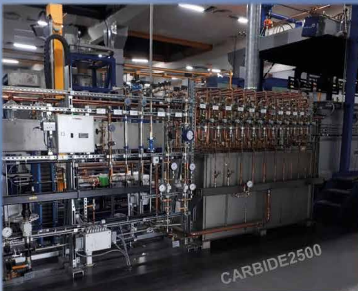
Pusher Type Plants for the Carburization of Tungsten, Tantalum and for Carbon Graphitization
