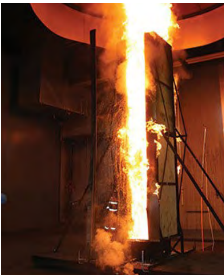
Fig. 3 “Code-compliant” cladding system failing 4.9m parallel panel test reaching peak heat release rate well in excess of 6000kW.
