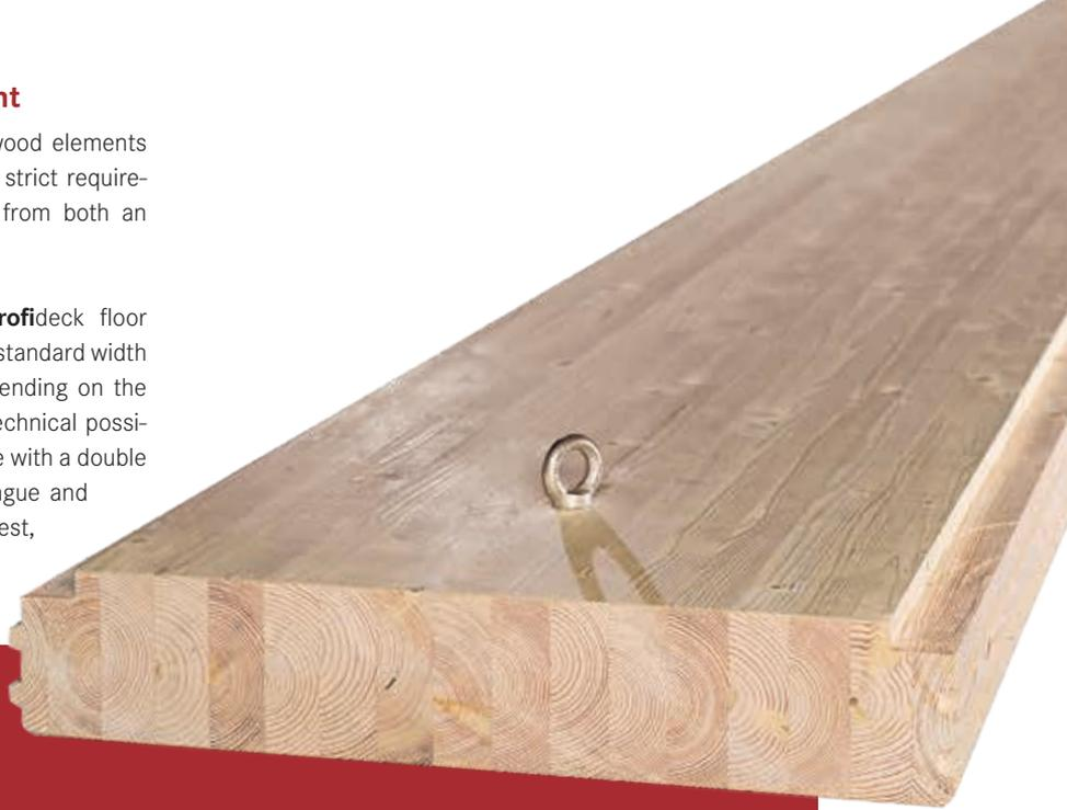
Note: in rooms that are heated to high temperatures, the joints between the elements may expand due to the shrinkage behaviour of wood. For this reason, element widths greater than 68 cm should be avoided.
