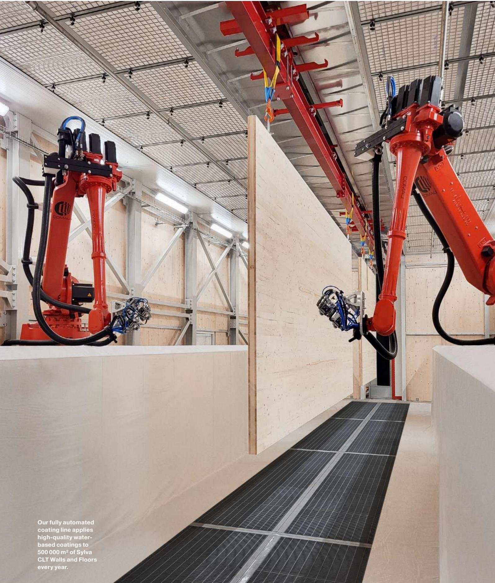
Our fully automated coating line applies high-quality water-based coatings to 500 000 m<sup>2</sup> of Sylva CLT Walls and Floors every year.
