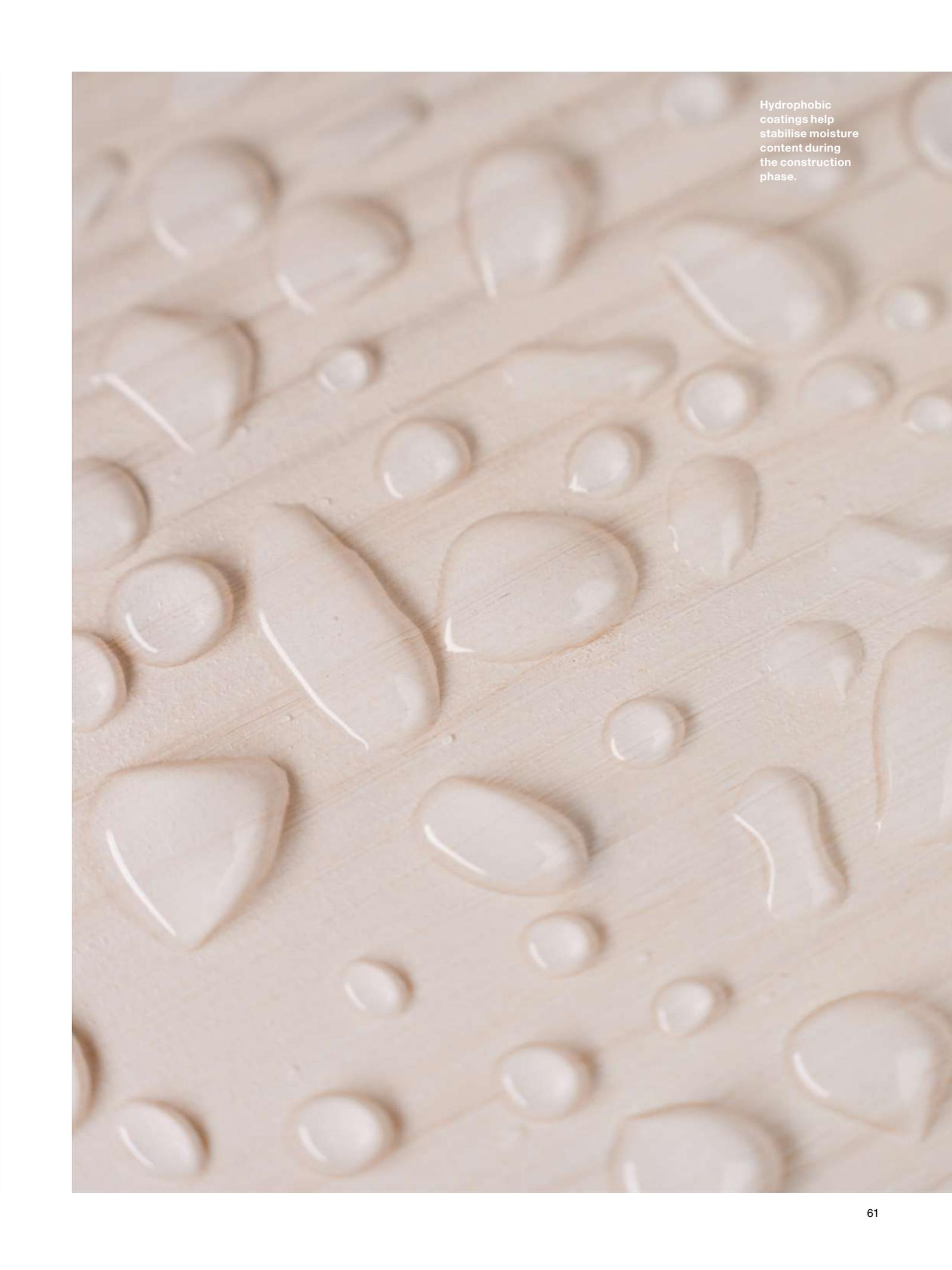
Hydrophobic coatings help stabilise moisture content during the construction phase.
