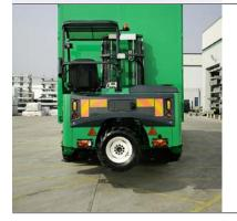
Truck with mounted forklift Driver authorization, certificate or similar license for "Forklift truck" required.
