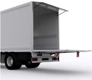
Truck with tail lift (hydraulic platform)
